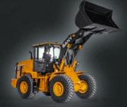
WHEEL LOADER SW305 Engine Deutz TCD 6.1 L6 Rated power 129 kW Bucket capacity 2,3 m<sup>3</sup> Operating mass 14 500 kg
